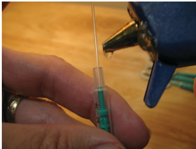
Figure 3. Hot Glue Added to Capillary Tube Base
